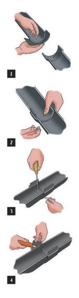
Note: When carrying out jointing or installation work on cast iron gutters, always check for any slight damage including paint chips and cut ends and if necessary use the appropriate touch up paint to ensure a complete covering.
